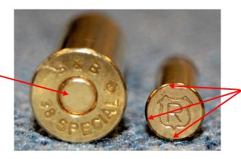
An RF cartridge is initiated by being struck anywhere on the rim of the case.
